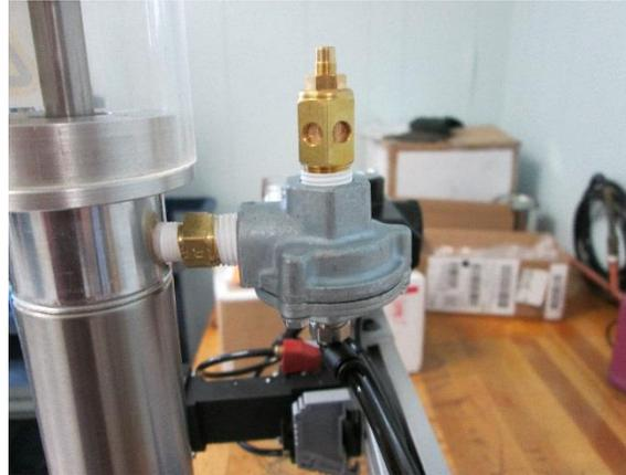
Adjusting your speed control mufflers can be done with a flat head screw driver and wrench. Turning the screw clockwise will cause that given direction of the press to slow. Inversely turning the screw counter clockwise will cause the press to move quicker in that direction.
